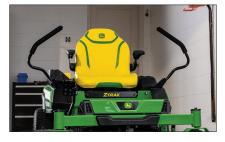
**Intuitive Controls:** Integrated park brake is activated when the control levers are pushed outward. Power button easily turns on machine.
