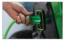
**On-Board Charging:** Just plug in a standard extension cord when you are done mowing and walk away. The Smart Charge Technology prevents over charging and maintains battery life.
