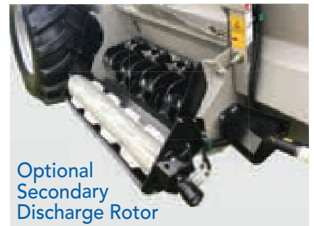
1.4m Wide Discharge Rotor With Hardox Bolt On Wear Plates
