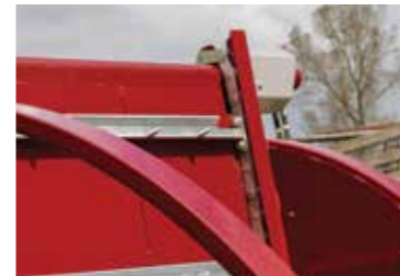
High-tensile 6mm folded channel tine bars have super aggressive tapered teeth to tear and release tightly baled feed. Bolted to 3" 15000lb solid pin chain
