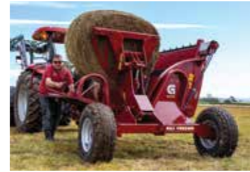
The controlled loading headstock can be paused above the feed bed for easy removal of net and wrap
