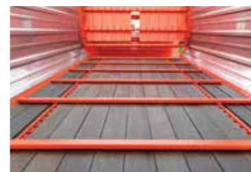
The durable hardwood floor and stainless steel sides protect against the corrosive effects of silage
