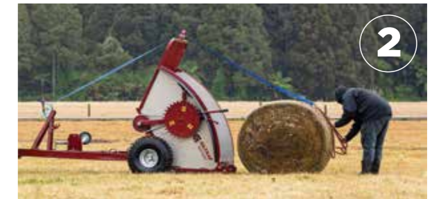
Release the winch and tilt the cradle onto the ground. Attach the two bale hooks to the winch stop. Using the hooks pull the stop out and over the back of the bale and push the hooks into the lower part of the bale
