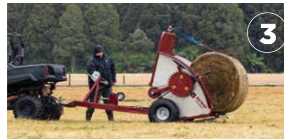
Begin to wind the geared winch which in turn will roll the bale into the cradle. When the bale enters the Bale Buggy, its weight will over-centre and the cradle will fall back into its transport position. Finish winding the stopper to its stopper and re-stow the hooks
