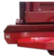
Autoshift ram extends the conveyor 200mm
