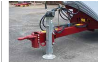
The swivel tow hitch can be adjusted for drawbar height. Complete with jack stand
