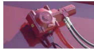
Gearbox elevator drive
