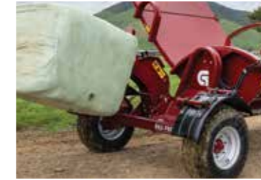
The extra wide 2.2m wheel track keeps the RS2 feeder stable on rough ground and hills
