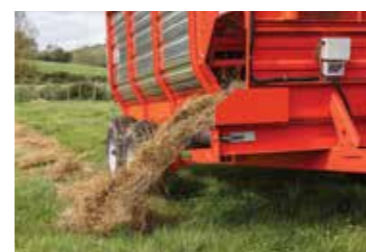
Easily adjustable load sensing rate control and conveyor speed lets you set the feed rate and control where the feed lands on the ground
