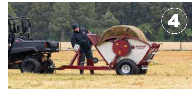
When you get to the paddock you want to feed out in, engage the ground wheel drive and you are read to go feeding. The bale will gently unroll over the back of the Bale Buggy at a ratio of 3:1 slower than your ground speed
