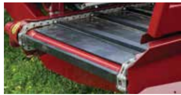
Chain and slat feedout conveyor
