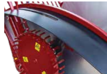
A polyethylene guard is fitted to ensure feed does not get caught in the chains or the drive mechanism
