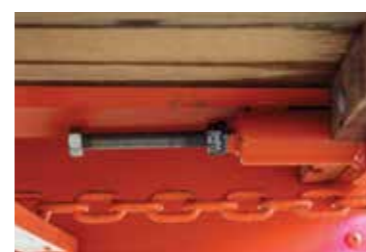
Floor and elevator chains are easily tensioned with stainless steel chain adjusters that won't corrode and seize
