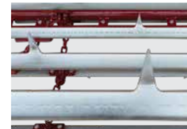
The teeth on the bars are offset to ensure even feedout of the bale. They are also tapered to release the feed easily
