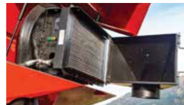
Heat exchanger keeps air flow dry
