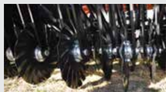
400mm opening turbo tilth discs for cutting through heavy trash
