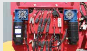
Mechanical gearboxes or high torque DC motor drives are easily adjustable and have infinitely variable sowing rate control
