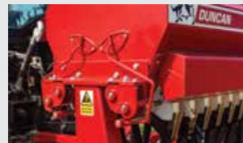
Adjustable flaps control the outlet flow
