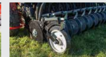
Press wheel following the double discs
