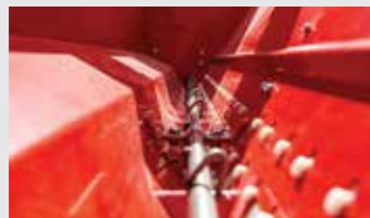
Stainless steel agitator shaft eliminates compaction and bridging, and improves the flow of fertiliser and seed
