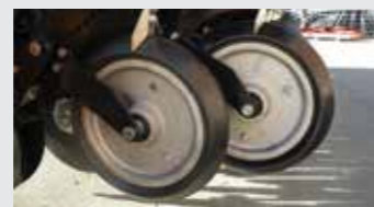
Adjustable wheels for closing the slot and controlling the depth
