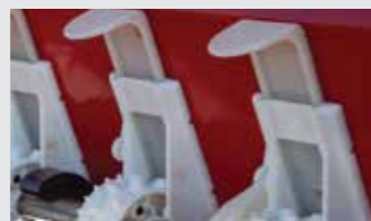
Shutter slides at the top of each metering device are used to control the seed flow and can also be used to shut off a seed row if required
