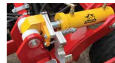
Depth adjustment on rams
