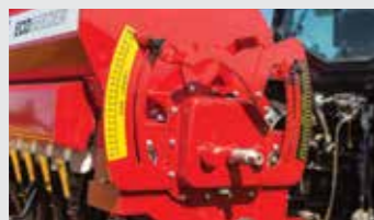
Mechanical gearboxes or high torque DC motor drives are easily adjustable and have infinitely variable sowing rate control
