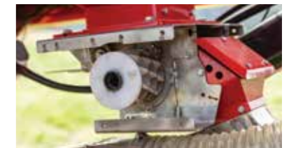
Stainless steel Amazone style metering system in both hoppers
