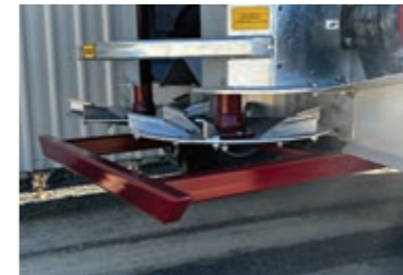
Spinner impact guard - reduces damage to spinners when operating in undulating areas or reversing
