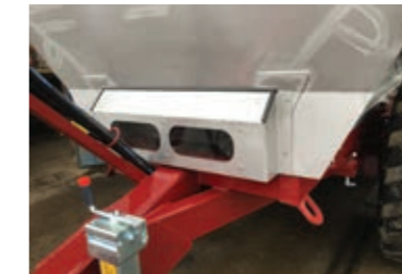
Front belt cover - protects belt from mud and debris thrown from the tractor during travel and reduces the possibility of product contamination
