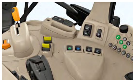
AutoPowr on the right-hand console with electrical SCVs
