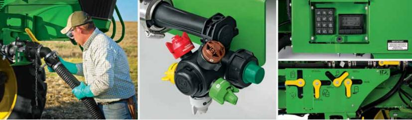
Exclusive Load Command<sup>™</sup> system (above left) dramatically cuts loading time on the R4045 Sprayer only. Load the 4,500 L tank as fast as three minutes. System automatically disengages when your sprayer tank is full. Plus, there's reduced risk of any product exposure.
