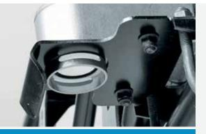
Add BoomTrac Pro<sup>™</sup> for automatic boom-height control. By maintaining correct boom height to target, you'll see improved application accuracy and efficiency, spray coverage and drift management. The boom height adjusts easily from 483 mm (19 in.) up to 2,337 mm (92 in.) to fit your needs.
