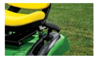
The convenient mower deck lift lever
